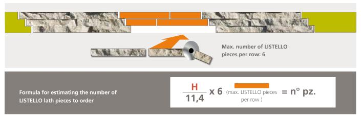
H Height (in cm) of wall between RIGO CORNERS / 11,4 Height (in cm) of the flat RIGO PANEL / 6 Max. number of LISTELLO RIGO pieces per row.
